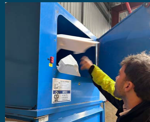
Jared Sherwin operating the Polystyrene Compactor
