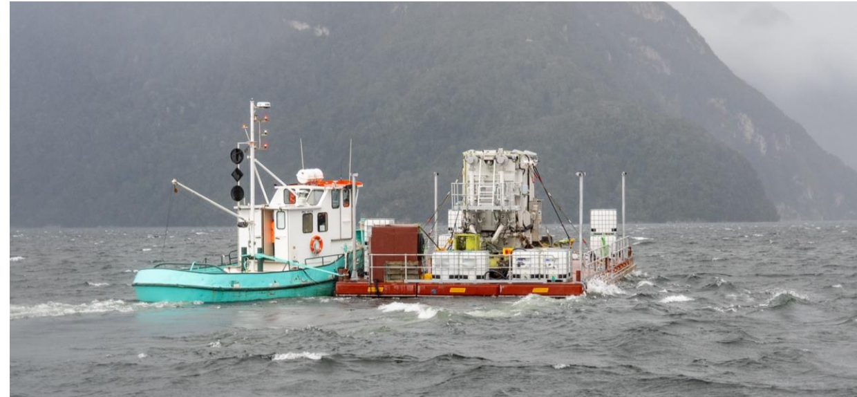
Transportation of a transformer across Lake Manapōuri
