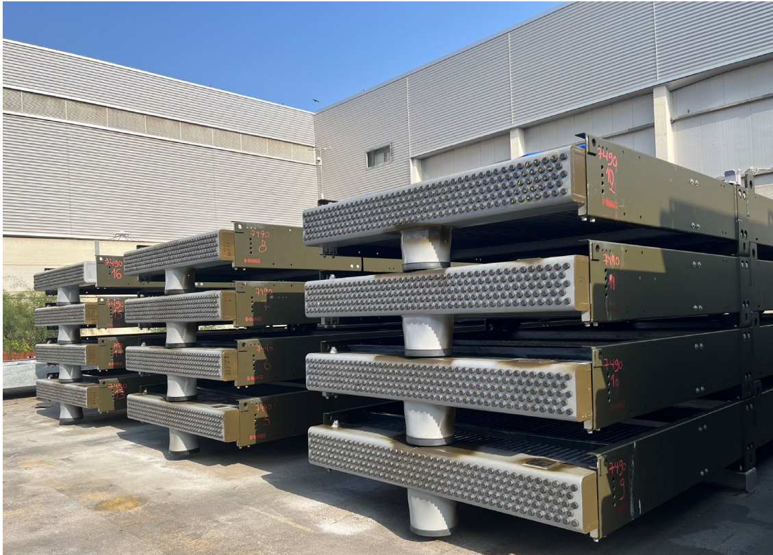
Air-cooled condensers for OEC5
