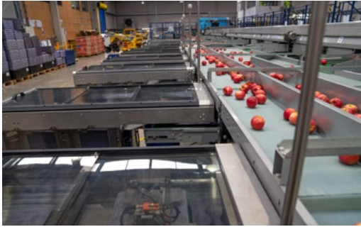
Tray de-nesting machines, part of the Whakatu packhouse automation project
