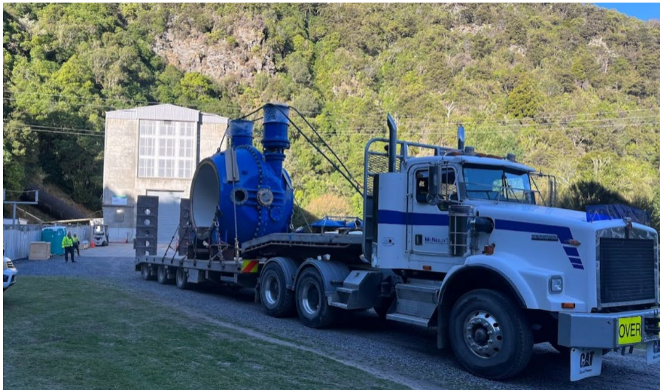
The 30 Ton, 70-year-old Main Inlet Valve returning to Waipori 3 Station following a complete overhaul.
