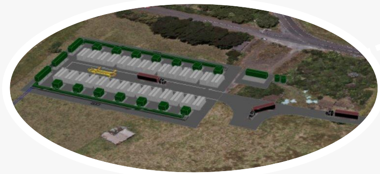
Image depicts battery megapacks, transformers, switchrooms, auxiliary facilities and access road at Glenbrook the site.
